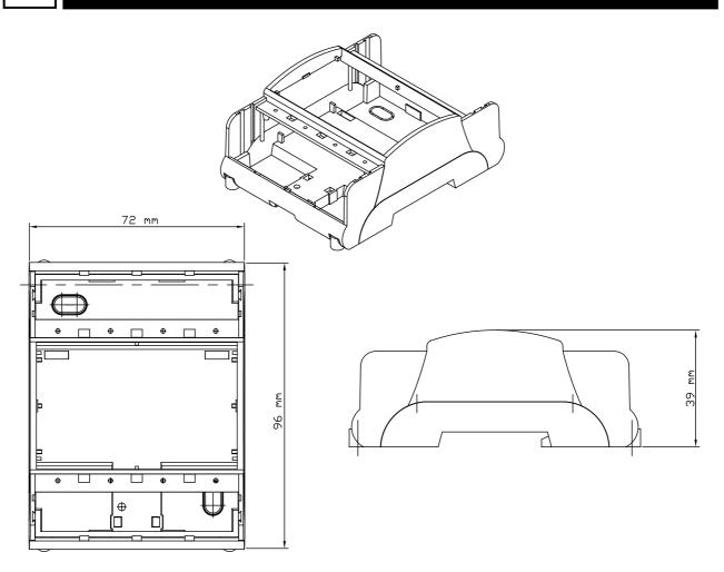
PAW-SERVER-PKEA can be installed in a standard DIN rail.
