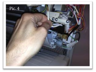
4) Insert the CAB-SERV connector into the CN-CNT plug on the Indoor PC Board (pic. 5, 6).
